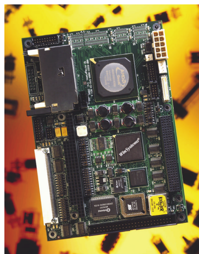
Figure 4 Featuring the AMD GX500 processor with integrated L1 cache, the EPX-GX from WinSystems offers a wide variety of I/O and network connectivity.
